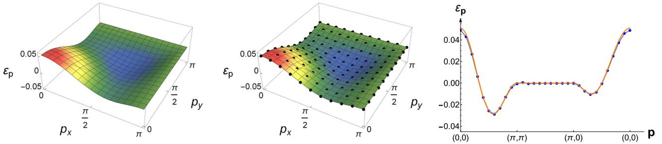
FIG. 1. Comparison between  $\varepsilon(\mathbf{p})$  from Eq. (18) (left) and the dispersion obtained from exact diagonalization (ED) for  $6 \times 6$  lattice sites with one fermionic dimer and twisted boundary conditions (middle) for  $J = V = 1$ ,  $v_1 = t_2 = -t_1 = 1$  and  $\delta t_3 = -0.02$ . Right: corresponding line cut through the Brillouin zone [blue line with dots: ED, orange line: Eq. (18)].
