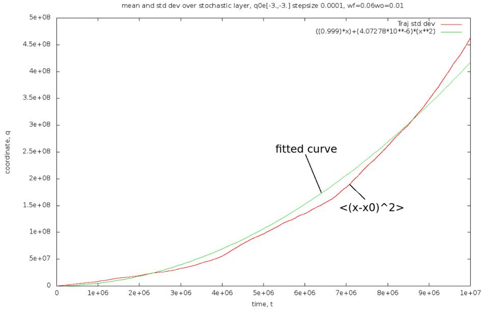
Figure 3.2: fit for  $\omega_f = 0.1 \cdot \omega_0 = 0.01$ : fit of  $\langle(\Delta x)^2\rangle = 0.999 \cdot t + 4.07 \cdot 10^{-6} \cdot t^2$
