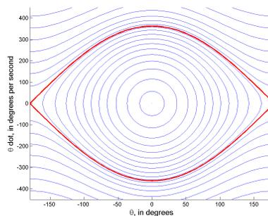
Figure 2.1: Separatrix of harmonic oscillator [26]
