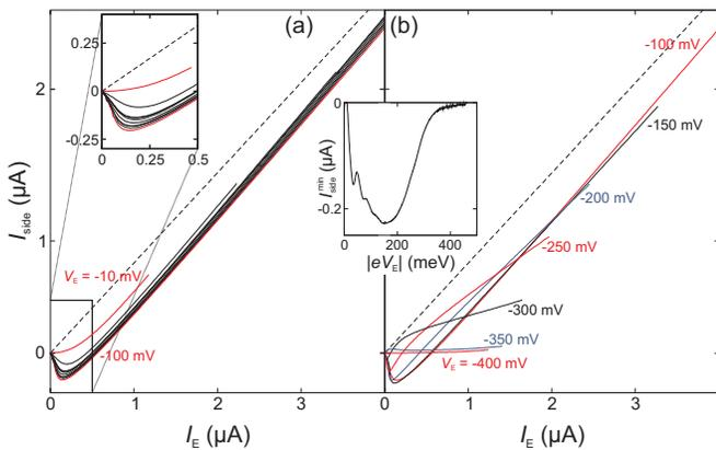
FIG. 4: (Color online)  $I_{\text{side}}$  as a function of injected current  $I_E$  for  $|V_E| \leq 100$  mV (spacing 10 mV) in (a) and  $|V_E| \geq 100$  mV in (b). Dashed straight lines represent ohmic behavior (see main text). The central inset plots  $I_{\text{side}}^{\text{min}}$  vs the energy of the injected electrons  $|eV_E|$ .
