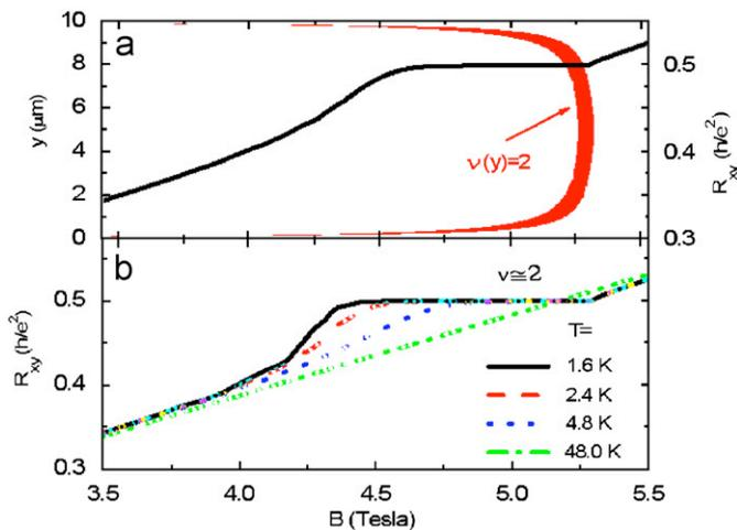
Fig. 1. (a) Calculated position of the incompressible strip at  $\nu = 2$  in a  $10 \mu\text{m}$  wide Hall bar as a function of the magnetic field. For the calculation we used  $k_B T/E_F^0 = 0.02$  and assumed an average electron density of  $3.79 \times 10^{11} \text{ cm}^{-2}$ . Also shown is the Hall resistance  $R_{xy}$  (black line) calculated for the same conditions. (b) Calculated  $R_{xy}$  as a function of magnetic field, at various temperatures.
