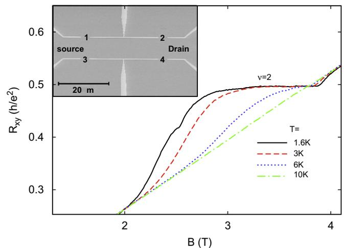
Fig. 2. Measured Hall resistance  $R_{xy}$  of a gate defined high mobility Hall bar for different temperatures in the vicinity of  $\nu = 2$ . The inset shows a scanning electron micrograph of the samples surface. Light gray areas are metal gates used to define the Hall bar with a width of  $10 \mu\text{m}$ .
