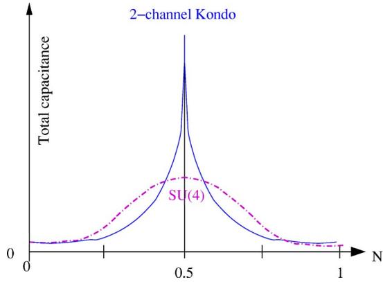
FIG. 13. (Color online) Sketch of the capacitance peaks (at zero temperature) for our setup with almost symmetric junctions (dashed line) compared to those in the original Matveev problem (full line) (Ref. 9)
