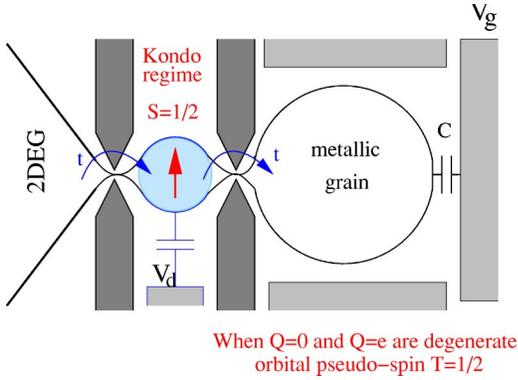
FIG. 1. (Color online) Schematic view of the setup. A micrometer scale grain (or large dot) is weakly coupled to a bulk lead via a small dot in the Kondo regime, which acts as an  $S = 1/2$  spin impurity. The charges of the grain and the small dot are controlled by the gate voltages  $V_g$  and  $V_d$ , respectively. The auxiliary voltages can be used to adjust the tunnel junctions.
