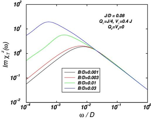
FIG. 6. (Color online) The orbital spin  $T^z$  susceptibility for different values of the external magnetic field  $B$ . The low-energy physics consists of a Fermi liquid regardless of  $B$ , but the symmetry is reduced for large magnetic fields to  $SU(2)$  (for the orbital space) and the Kondo energy scale is also reduced.
