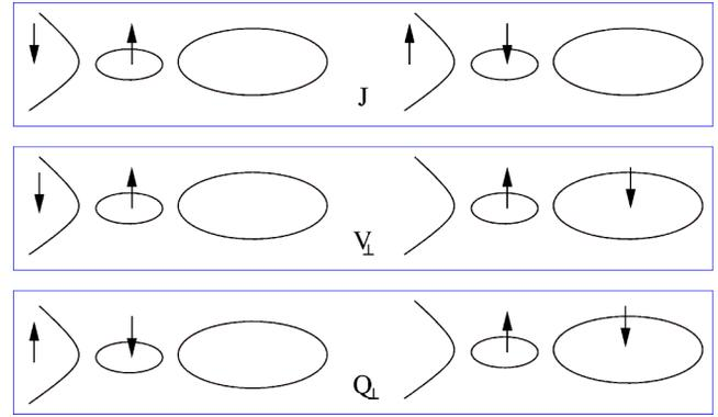
FIG. 2. (Color online) Couplings involved after the Schrieffer-Wolff transformation:  $J$  refers to *pure* spin-flip processes involving the  $S=1/2$  spin of the small dot,  $V_\perp$  to *pure* charge flips from the lead to the grain, and  $Q_\perp$  to exotic spin-flip-assisted tunneling, i.e., mixing the charge fluctuations of the grain with the screening of the  $S=1/2$  spin of the small dot.
