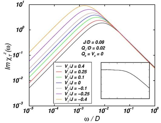
FIG. 5. (Color online) The orbital spin  $T^z$  susceptibility for different values of  $V_\perp$ . In all cases the susceptibility shows a typical SU(4) Fermi liquid state at  $\omega = T_K^{\text{SU}(4)}(V_\perp)$ . Inset: As a comparison we plot the same quantity for the two-channel Kondo model. Furthermore, we can clearly observe that  $T_K^{\text{SU}(4)}$  markedly decreases for lower values of  $U$ , i.e., by making the small dot larger and larger (Ref. 46), meaning  $V_\perp/J < 0$ .
