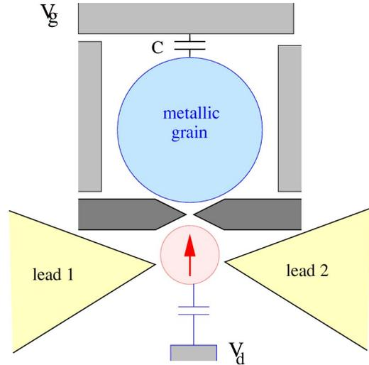
FIG. 14. (Color online) Another mesoscopic double-lead setup, a candidate for the  $SU(4)$  model. This could be equally performed with vertically coupled dots (Ref. 29).
