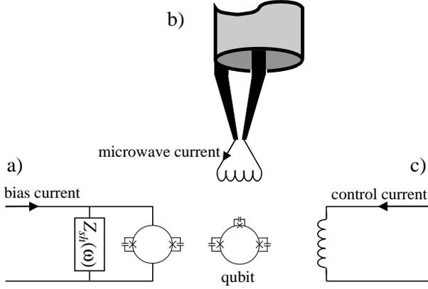
**Fig. 1.** Experimental setup for measurements on a Josephson persistent-current qubit. The qubit (center) is a superconducting loop that contains three Josephson junctions. It is inductively coupled to a DC-SQUID (a), and superconducting control lines for applying magnetic fields at microwave frequencies (b) and static magnetic fields (c). The DC-SQUID is realized with an on-chip shunt circuit with impedance  $Z_{sh}$ . The circuits a)–c) are connected to filtering and electronics (not drawn).
