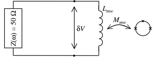
**Fig. 8.** Circuit model for coaxial line that is inductively coupled to the qubit. The coaxial line is modeled as a 50  $\Omega$  impedance that is shorted near the qubit with an inductance  $L_{mw}$ . The qubit is coupled to this short with a mutual inductance  $M_{mw}$ . The noise that couples to the qubit results from Johnson-Nyquist voltage noise  $\delta V$  from the circuit's total impedance  $Z_t$ , formed by a parallel combination of the 50  $\Omega$  impedance and  $L_{mw}$ .
