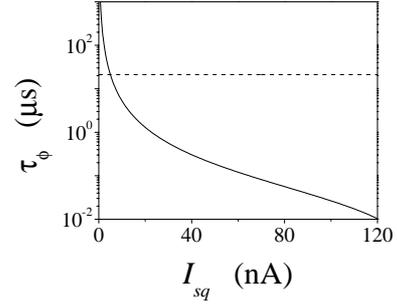
**Fig. 7.** The dephasing time (42) as a function of the bias current  $I_{sq}$  through the SQUID (solid line). The dashed line shows  $\tau_\phi$  for  $I_{sq} = 5$  nA, a typical minimum value for the effective bias current for a SQUID with a few percent asymmetry between its junctions. At this point  $\tau_\phi = 131 \mu\text{s}$ , and  $\alpha = 1 \times 10^{-7}$ . Parameters are further as described in the caption of Figure 5.
