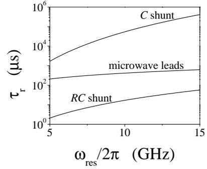
**Fig. 6.** Typical relaxation times due to the  $C$ -shunted SQUID, the  $RC$ -shunted SQUID, and coupling the microwave leads as a function of the resonance frequency at which the qubit is operated. The example of the microwave leads contribution is for a mutual inductance  $M_{mw}$  to the coaxial line of  $M_{mw} = 0.1$  pH. Parameters are further as described in the caption of Figure 5.
