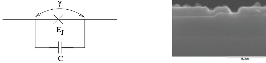
Figure 2.1: Left picture is an equivalent circuit diagram of a Josephson junction. The junction itself is depicted by a cross, and might be described as a junction that is shunted by a shunt capacitor  $C$ , reflecting the geometric capacitance between the electrodes.  $E_J$  is the Josephson energy defined in equation (2.3). The right picture is a SEM image of a Josephson junction (TU Delft). A thin oxide layer is fabricated in-between the aluminium layers.
