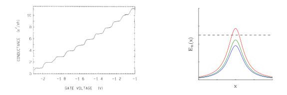
Figure 1.4.: Left: Measurement of the quantized conductance in the original paper by Van Wees et al. [2] from 1988. The height of the barrier is here reduced with increasing the gate voltage. Right: Graphical depiction of the channels leading to the conductance quantization. We sketched here a set of curves  $E_n(x)$  corresponding to different channels; the ones below the *E* line represent open channels, the one which intersects *E* is a closed channel.
