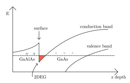
Figure 1.2.: Cut through the semiconducting layers of our GaAlAs-GaAs structure. The 2DEG (here depicted in red) formes at the junction between the layers.
