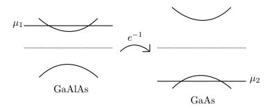
Figure 1.1.: Bandstructures of the semiconductors GaAlAs and GaAs. Note the different chemical potentials due to the respective doping.
