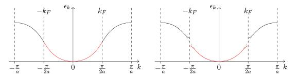
Figure 2: The left diagram shows the filled electron energy states (red) in the unperturbed system. The right diagram shows the opening of the gap in the energy spectrum due to lattice distortions and the resulting lowering of the electron energies.
