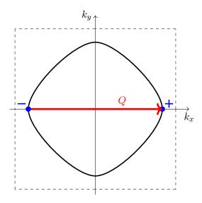
Figure 4: The CDW wave vector  $\mathbf{Q} = 2k_F$  connects two points on the Fermi surface with parallel tangents.
