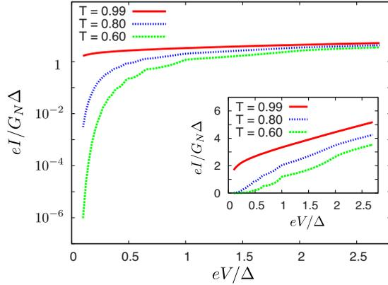
FIG. 3. (Color online) Current through a homogeneous multi-mode contact with high transmission between superconductors as a function of bias voltage, at zero temperature, on a logarithmic current scale. Inset: linear current scale.
