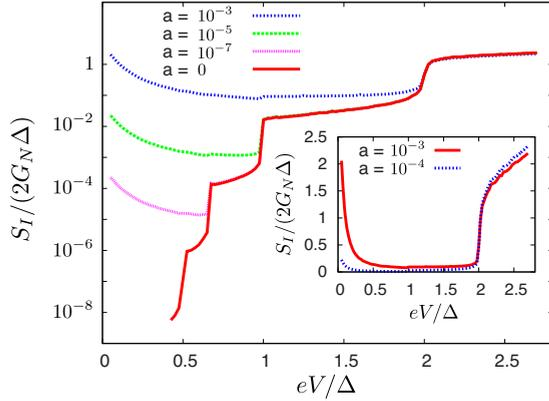
FIG. 9. (Color online) Noise  $S_I$  on a logarithmic scale as a function of bias voltage, at zero temperature, for a rough superconducting tunnel junction characterized by the transmission eigenvalue distribution  $\rho(T) = a\delta(T - T_1) + (1 - a)\delta(T - T_2)$ ,  $T_1 = 0.986$  and  $T_2 = 0.01$ . The different curves refer to different pinhole fractions  $a$  within all transport channels. Inset: linear noise scale.
