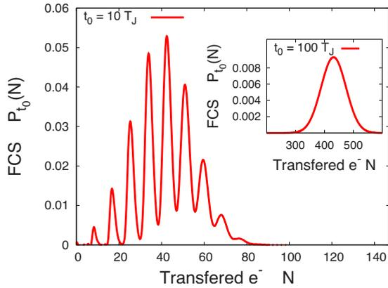
FIG. 10. (Color online) FCS for a transport channel between superconductors with transmission  $T=0.936$  and voltage bias  $eV=0.3\Delta$  at measurement time  $t_0=10T_J$ . Inset: measurement time  $t_0=100T_J$ .
