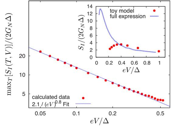
FIG. 8. (Color online) Maximal noise  $\max_T[S_I(T, V)]$ , optimized with transmission as a parameter, as a function of bias voltage on a double-logarithmic scale for a homogeneous contact between superconductors. The calculated data using the full expression, Eq. (1), are fitted using the given power law. Inset: comparison of the noise results calculated for a  $T=0.97$  homogeneous contact between superconductors as a function of bias voltage using either the full expression or the toy model.
