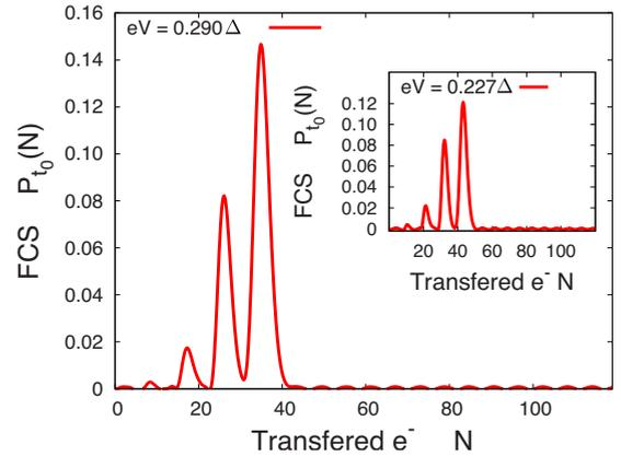
FIG. 11. (Color online) FCS for a transport channel between superconductors with transmission eigenvalue  $T=0.99$  and voltage bias  $eV=0.290\Delta$ . Inset:  $eV=0.227\Delta$ . The measurement time is  $t_0=4T_J$ .
