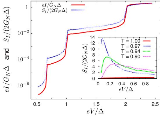
FIG. 5. (Color online) Noise and current as a function of bias voltage, at zero temperature, for a homogeneous superconducting tunnel junctions with transmission eigenvalue  $T=0.01$ . Inset: noise characteristics for junctions with large transmission.
