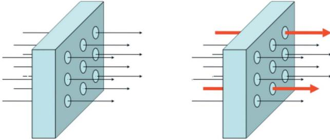
FIG. 1. (Color online) Schematic of the oxide layer of a Josephson Junction. Several transport channels are indicated. The arrow thickness corresponds to the respective transmission eigenvalue. Left: schematic of an ideal Josephson tunnel junction. The transmission of all channels is small. Right: considered *rough Josephson tunnel junction*, i.e., a tunnel junction including some high-transmission channels, so-called pinholes.
