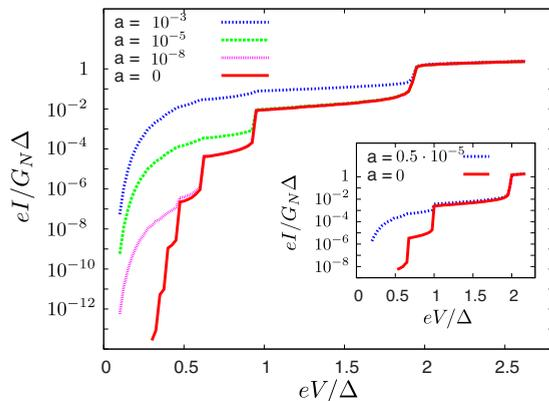
FIG. 4. (Color online) Leakage current on a logarithmic scale as a function of bias voltage, at zero temperature, for a rough superconducting tunnel junction with transmission eigenvalue distribution  $\rho(T) = a\delta(T-T_1) + (1-a)\delta(T-T_2)$ ,  $T_1=0.6$ , and  $T_2=0.01$ . Inset:  $T_1=0.6$  and  $T_2=0.003$ . The different curves refer to different pinhole fractions  $a$  within all transport channels.
