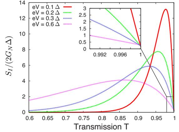
FIG. 6. (Color online) Noise  $S_I$  as a function of transmission eigenvalue  $T$  for a homogeneous superconducting tunnel junction where the bias voltage is set as parameter. Inset: enlargement around  $T=1$ .
