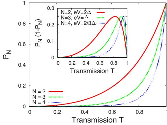
FIG. 7. (Color online) Toy-model probability  $P_N$  to transfer  $N$  charges at a time as a function of transmission eigenvalue  $T$ . Inset: expression  $P_N(1-P_N)$ , that occurs as a term in the second cumulant [Eq. (8)], as a function of transmission eigenvalue  $T$ .
