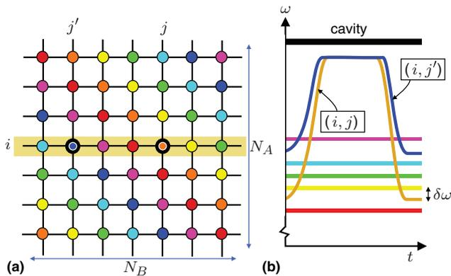
Fig. 1: (Colour on-line) Schematic cavity grid setup. (a) The 2D cavity grid, with qubits depicted as circles and cavities shown as lines. Qubit  $(i, j)$  sits at the intersection of cavities  $i$  and  $j$ . Colors distinguish the transition frequencies, which differ within any column or row (in the “idle state”). (b) A two-qubit operation is induced by tuning two qubits into mutual resonance to exploit the cavity-assisted dispersive coupling.
