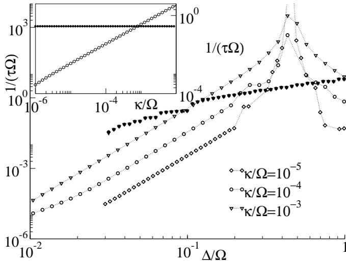
Figure 3.6: Comparison of dephasing / discrimination rates. Open symbols:  $1/(\tau_\phi\Omega)$  and filled symbols:  $1/(\tau_{\text{discr}}\Omega)$ . Here  $\nu = 1.1\Omega$ ,  $\overline{F}_0 = 200$  and  $\hbar\Omega/(k_B T) = 2$ . Inset: dependence on  $\kappa$  for  $\Delta/\Omega = 0.1$ .
