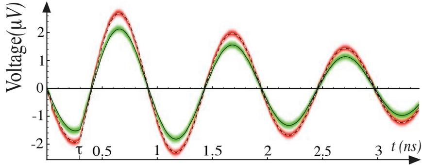
Figure 5.4: Probability distribution of output voltage (density plot, dark color indicates high and white low density) and expectation value of momentum for the two qubit states  $|\downarrow\rangle$  (dashed, red) and  $|\uparrow\rangle$  (continuous, green). Here  $\Omega/(2\pi) = 0.97$  GHz,  $\Omega/\kappa = 20$ ,  $w = \Omega$ ,  $\Omega\tau = 1.83$ ,  $\delta\tau = 0.015$ ,  $\gamma\tau = 3$ ,  $T = 30$  mK. The values of the circuit parameters are given in section 5.6.2.
