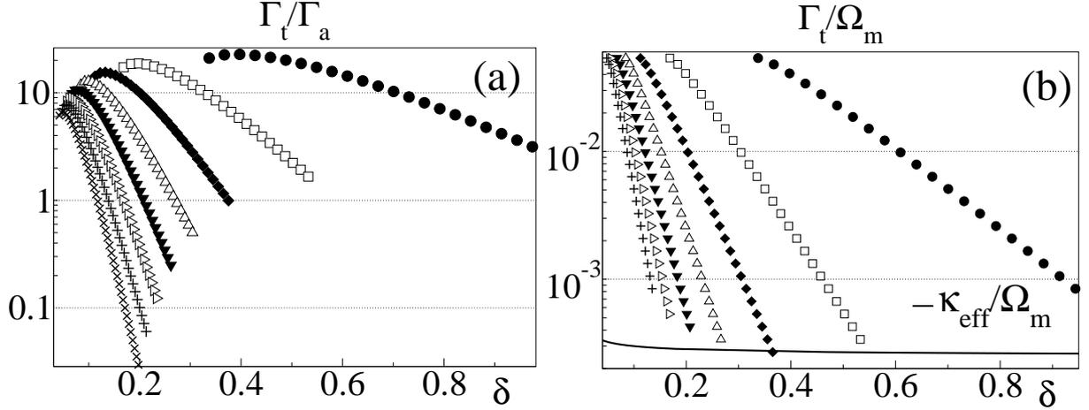
Figure 6.5: (a) The ratio of tunneling and activation rates from the small well at the avoided level crossings. (b) Corresponding tunneling rates compared to  $\kappa_{\text{eff}}$  (where  $\Gamma_t/\Gamma_a > 1$ ). Driving frequency sweep at  $F_0 = 0.7F_c(\nu)$ ; Values of  $\Omega$  (in GHz): 1( $\bullet$ ), 2( $\square$ ), 3( $\blacklozenge$ ), 4( $\triangle$ ), 5( $\blacktriangledown$ ), 6( $\triangleright$ ), 7(+), 8( $\times$ ), at parameters specified in text.
