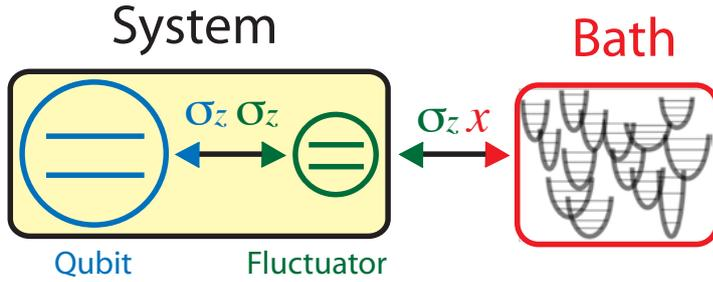
Figure 8.1: Illustration of the coupled system qubit-fluctuator-bath.
