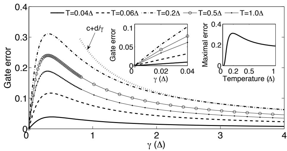
Figure 8.5: Gate error versus TLF rate  $\gamma$  for various temperatures for a long optimized pulse ( $t_g = 60/\Delta$ ,  $E_2 = 0.1\Delta$  and  $\Lambda = 0.1\Delta$ ). A high  $\gamma$  fit with  $c + d/\gamma$  is also pictured. The left inset is a magnification of the low  $\gamma$  part of the main plot and reveals the linear behaviour. The right inset shows the maximum of the curves versus temperature.
