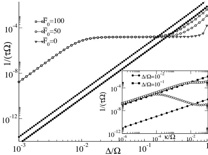
Figure 3.5: Comparison of dephasing / measurement rate. Open symbols:  $1/(\tau_\phi\Omega)$  and filled symbols:  $1/(\tau_m\Omega)$ . Here  $\nu = 2\Omega$ ,  $\kappa = 10^{-4}\Omega$  and  $\hbar\Omega/(k_B T) = 2$ . Inset: dependence on  $\kappa$ ,  $\bar{F}_0 = 200$ . The crossings, conflicting with the quantum limit [5], are signaling the limits of the Born approximation, as described in text.
