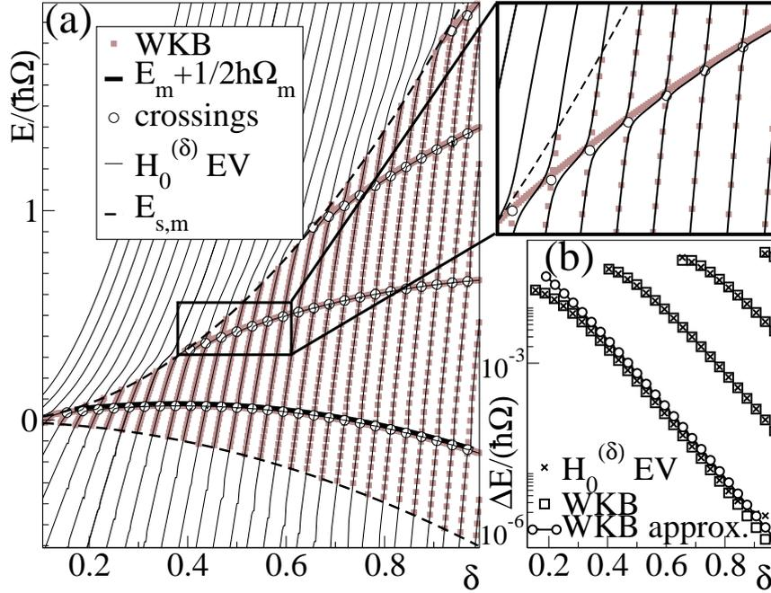
Figure 6.3: (a): Quantized energies: eigenvalues (EV) of  $\hat{H}_0^{(\delta)}$  versus WKB.  $\hat{H}_0^{(\delta)}$  was represented in the number state basis considering  $2N$  levels. (b): Tunneling-induced energy splittings at level crossings. Frequency sweep at  $m\Omega/\hbar = 2$ ,  $\beta = m\Omega^2/24$ ,  $\kappa\omega_c/\Omega^2 = 0.1$  and  $F_0 = 0.5F_c(\nu)$ .
