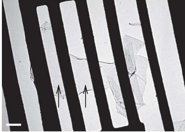
Figure 3: A freely suspended graphene flake attached to a micrometer-sized metallic scaffold. The regions indicated by the arrows are monolayer graphene. On the righthand side there is a folded part of the sheet visible. The scale bar is 500nm large.
