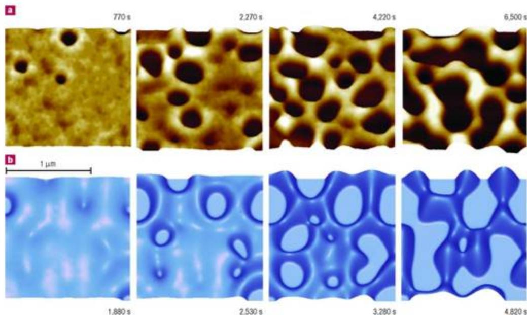
a) AFM recording of an experiment with a 3.9 nm polystyrene film on an oxidized Si wafer. b) Simulation. Nature materials Vol 2 JAN 2003 Jürgen Becker et al.
