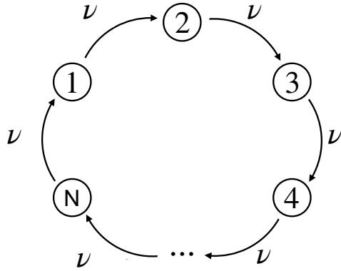
We consider a continuous-time Markov process on a ring of  $N$  discrete states. Transitions occur only from  $i \rightarrow i+1 \bmod N$  at constant rate  $\nu$ . This is a minimal model of a non-equilibrium steady state with persistent probability currents.
