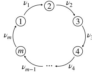
The individual transitions  $i \xrightarrow{\nu_i} (i+1)$  are assumed to be statistically independent. The reaction times  $T_i$  of each transition are random variables, which we assume to be distributed exponentially:
