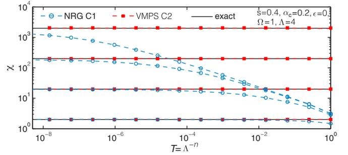
FIG. 2. DHO susceptibility  $\chi(T)$  as function of temperature, computed by NRG on C1-RWCs (circles) and by VMPS on C2-RWCs (squares), for  $\alpha = 0.1, 0.19, 0.199$ , and  $0.1999$  (from bottom to top). Solid lines show exact results.
