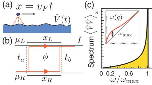
FIG. 1 (color online). (a) A single electron propagating at high energies feels a fluctuating potential  $\hat{V}(t)$ , as it interacts with the sea of other electrons. (b) Scheme of the Mach-Zehnder interferometer setup. (c) The fluctuation spectrum (at  $T = 0$  and  $\alpha > 0$ ). Inset: Plasmonic dispersion relation.
