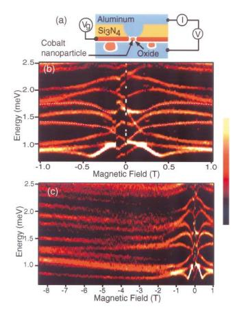
FIG. 1 (color). (a) Cross-sectional device schematic. (b),(c) Color-scale plots of dI/dV for tunneling resonances in a cobalt nanoparticle. The field is varied from positive to negative values, and dI/dV vs V is measured at each step. The maximum conductance is  $3 \times 10^{-9} \ \Omega^{-1}$ .
