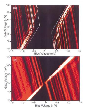
FIG. 3 (color). Color-scale conductance plots of a gated Co nanoparticle as a function of  $V_g$  and V. (a) Superconducting leads (H=0). (b) Normal-state leads (0.07 T). The maximum conductance is  $7\times 10^{-9}~\Omega^{-1}$  in (a) and  $3.5\times 10^{-9}~\Omega^{-1}$  in (b). The dashed lines in (a) indicate the expected evolution of the threshold peaks if the resonances did not involve nonequilibrium processes. The electron  $T\approx 90$  mK.
