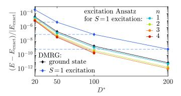
FIG. 2. Relative error in energy of the lowest-lying S = 1 excited state of the Haldane-Shastry model, computed using the *n*-site excitation Ansatz (circles), or using DMRG (blue diamonds). Black diamonds show DMRG results for the S = 0 ground state. The dashed-blue lines are guides to the eye.
