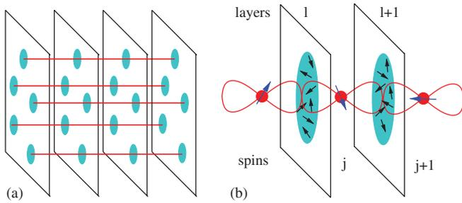
Fig. 1. (a) Layered lattice of spatially separated charges in planes and spins in chains. (b) A fragment of a chain with Kondo clouds formed as “shadows” in metallic layers.
